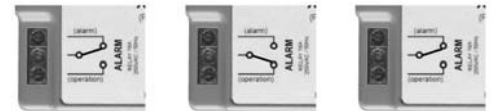
Power unit without power supply Power unit with power supply (operation) Power unit during alarm condition
