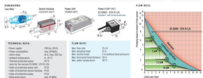
(Cooling capacity: 10 kW x 0.8 L/h = max. 8 L/h)
