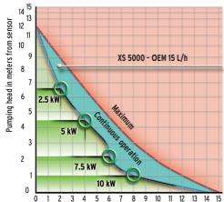
(Cooling capacity: 10 kW x 0.8 L/h = max. 8 L/h)
